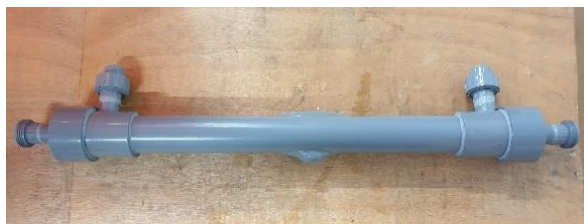
Figure 5-20: Damaged membrane module after placing it in a microwave cavity (center)
