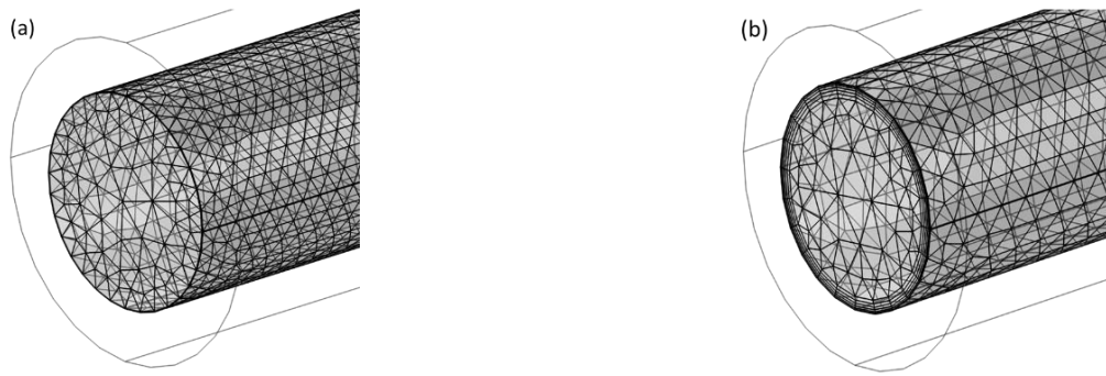
Figure 4-19: Meshing of the fiber lumen domain using two different configurations: (a)-Extremely Fine; (b)-Custom 2.
