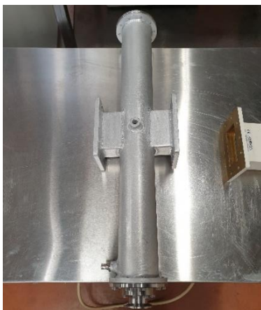
Figure 5-15: Microwave cavity for solvent preheating
