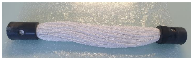
Figure 5-21: Hollow fibers of membrane module after stripping the PVC shell material
