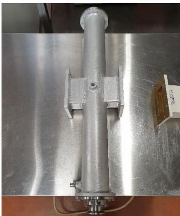
Figure 5-15: Microwave cavity for solvent preheating
