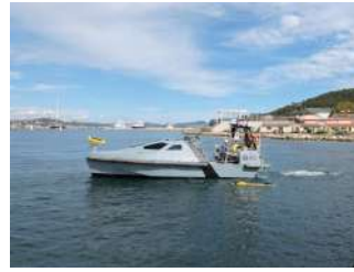
Figure 2.15. : Appareil de surface autonome de support Inspector 125.
