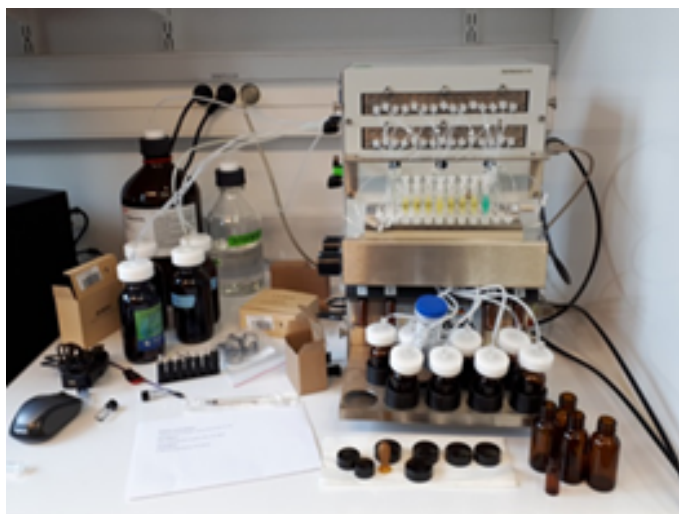
Figure 5.4: DNA synthesizer used for solid-phase synthesis of DNA and RNA oligonucleotides.
