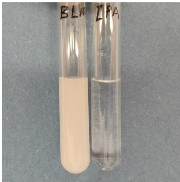
Figure 5.7. Mixture of benzaldehyde and BLM (left) and benzaldehyde and IPA (right)
