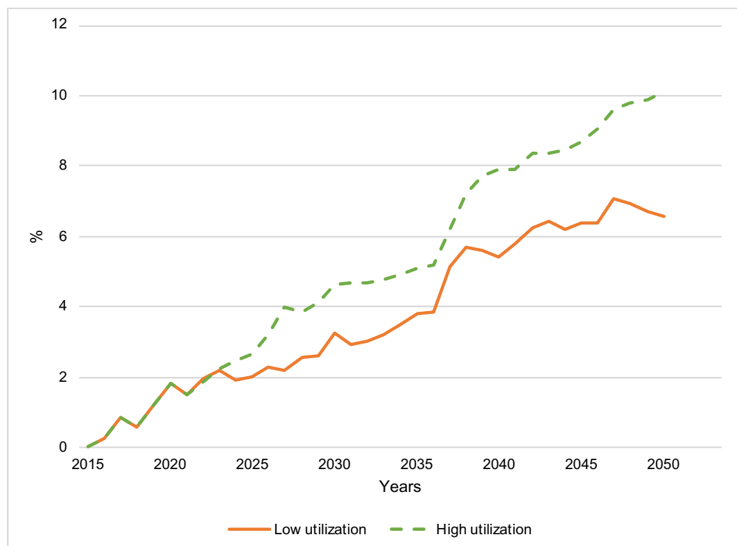
Fig. 10. Impact of resource dynamics modelling on estimated average unit production cost of geothermal electricity.
