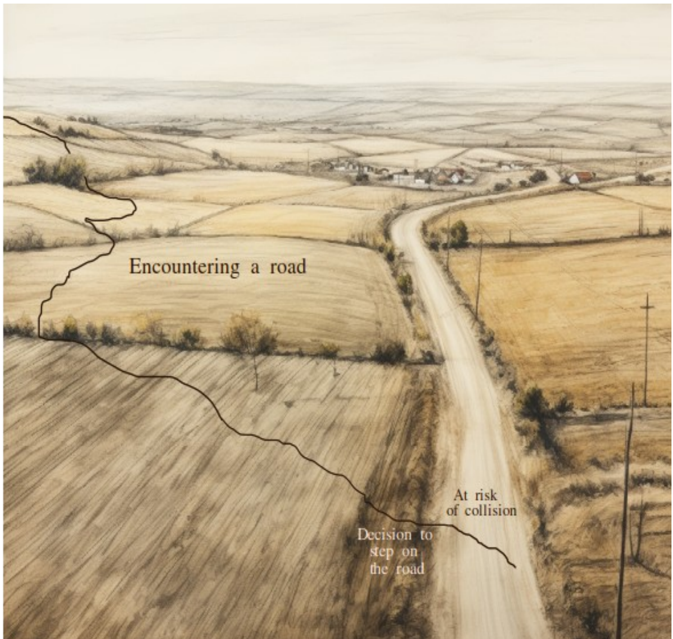
Fig. 6: Conceptual model of a wildlife-vehicle collision model. The probability of collision is the result of three consecutive steps: the probability to encounter a road, the decision to step on the road surface, and finally, the probability of a collision with a vehicle while on the road surface.
