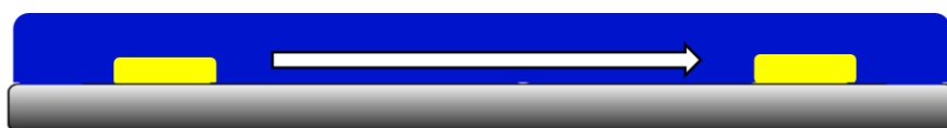
Scheme 1. Schematic view of simple chemiresistive devices. The arrow indicates the charge flowing pathway.
