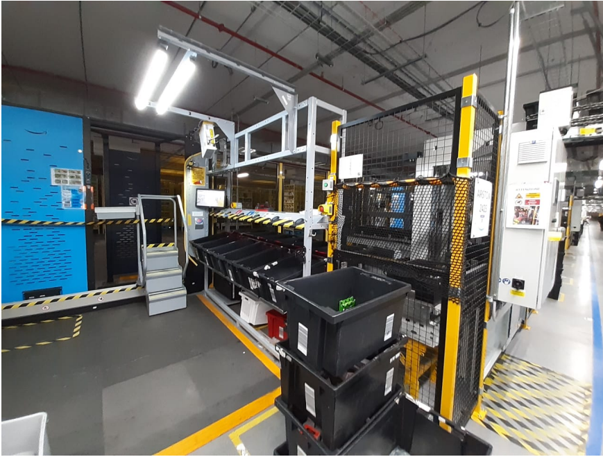
Figure 29 – Picking/Stowing Workstation in an Amazon Robotic FCs (Italy, 2023)
