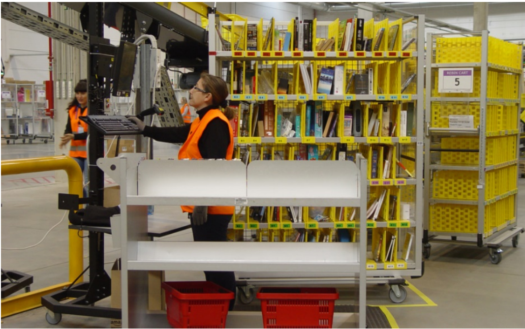
Figure 26 – A rebin workstation, FRA1, Germany (All About Lean 2019)
