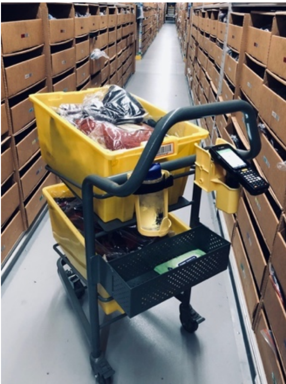
Figure 24 – A picking cart, with two totes and a scan
