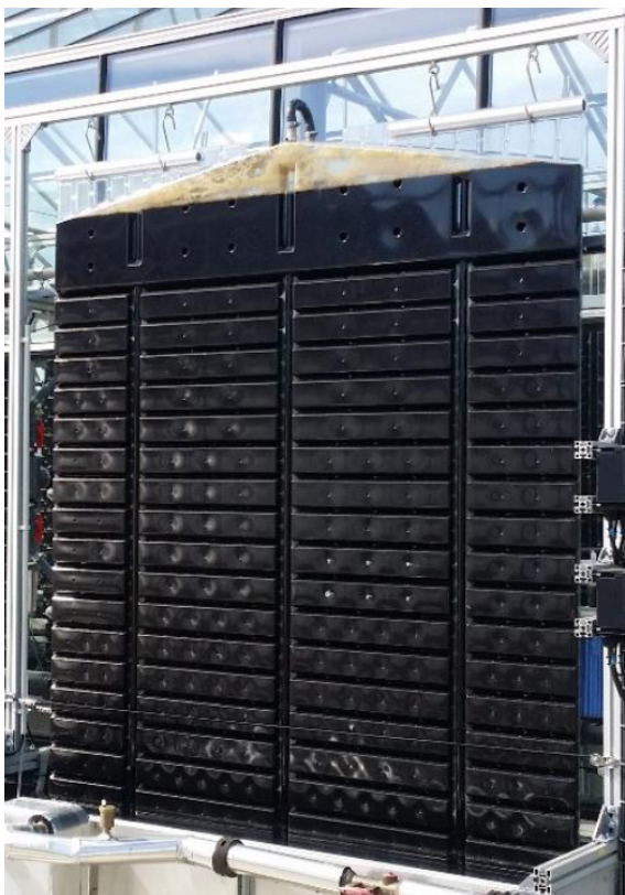
Figure 7.4: Flat panel photobioreactor where the microalgae were cultivated.
