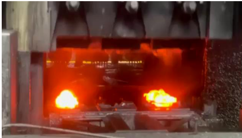
Figure 2 : Die forging at Stellantis Mulhouse.
