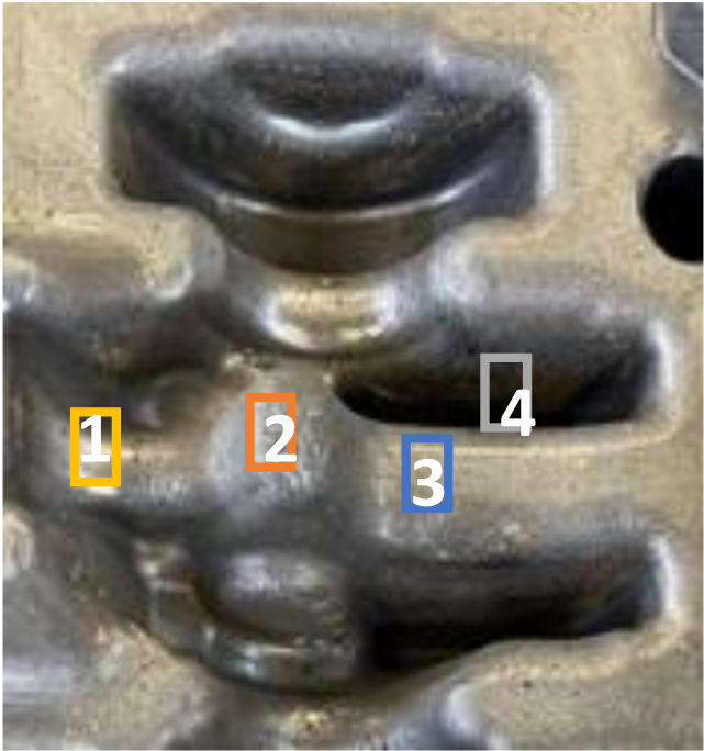
Figure 35: The selected zones: concave (1), convex (2), flat (3) and bottom of the engraving (4).
