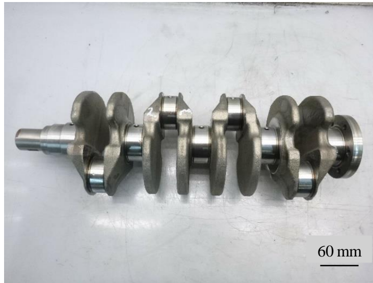
Figure 3: Crankshaft designed for four-cylinder petrol engines.
