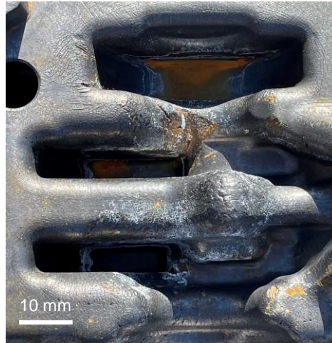
Figure 17: The presence of wear on the hot forging dies for crankshaft (20,000 cycles) at Stellantis
