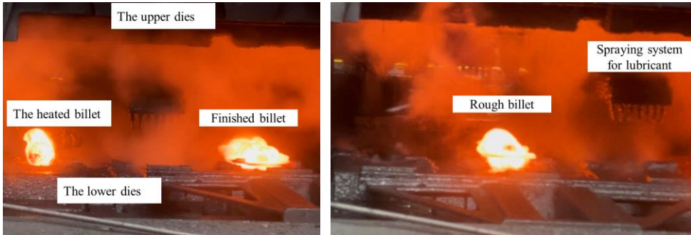
Figure 6: The 3 steps of the forging of the crankshaft on the mechanical press at Stellantis.
