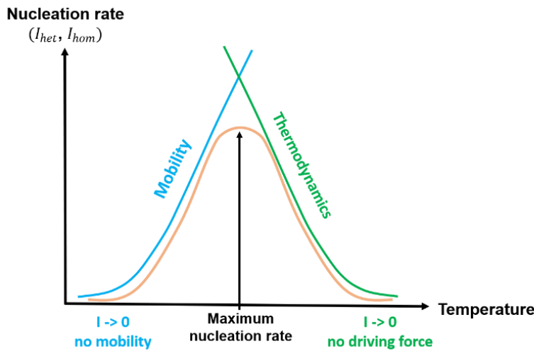
Figure I.4. Temperature dependence of the nucleation rate and its two contributions, i.e. molecular mobility and thermodynamic driving force.
