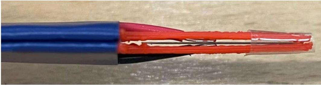
Figure 2.32. Illustration of using a sample holder to mount ME samples during measurements.
