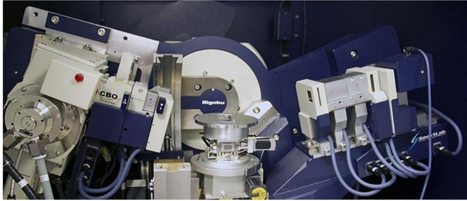
Figure 2.15. Rigaku Smartlab Diffractometer was utilized for the XRD measurements, in the laboratory INSP.
