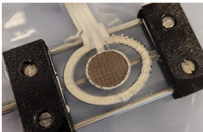
Figure 124. Example of ring-shaped electrode consumed in an electrolytic bath under tensile constraint. Picture by E. Neveux
