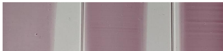
Figure 3-17: Optical macroscope images of P3HT:PC 61 BM np -BHJ deposited with bar coater with varying bar speed.
