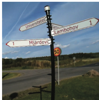
Figure 4.1 – A photo from an iPhone 3GS camera acquired during fast motion [Forssén 10]. The pole holding the signs is slanted instead of being straight.
