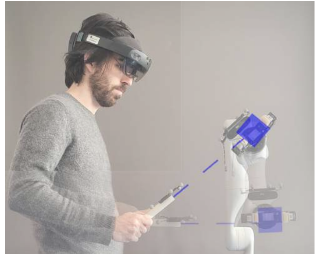
Fig. 1: The setup of the virtual link involves a virtual end-effector (represented by a blue square) connected to the user’s hand via a virtual link (illustrated by a dotted blue segment). This connection can optionally be visualized through an augmented reality headset. The length of the link can either remain rigid, which limits the workspace’s depth, as depicted here, or be reconfigured using an auxiliary velocity input device, creating a hybrid position/velocity controller. A nearby robot has its end-effector servoed to follow the desired end-effector position indicated by the virtual link.
