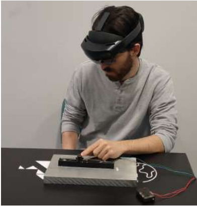
Fig. 4: View of a participant with the experimental set-up wearing the Microsoft HoloLens headset and manipulating the tangible interface.
