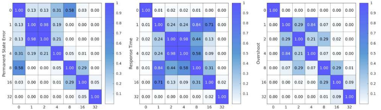
Fig. 8: pValues of the 2-by-2 Mann-Whitney-Wilcoxon tests. From left to right: the permanent state error, the response time and the overshoot. The higher the p-value, the bluer is the corresponding cell. White cells mean that the metrics are significantly separable for the two gains.
