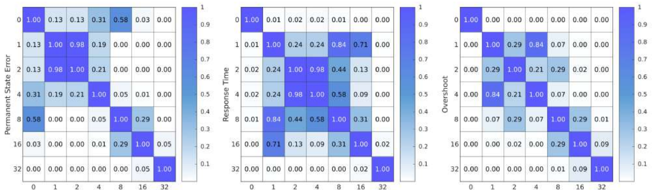
Fig. 10: pValues of the 2-by-2 Mann-Whitney-Wilcoxon tests. From left to right: the permanent state error, the response time and the overshoot. The higher the p-value, the bluer is the corresponding cell. White cells mean that the metrics are significantly separable for the two gains.
