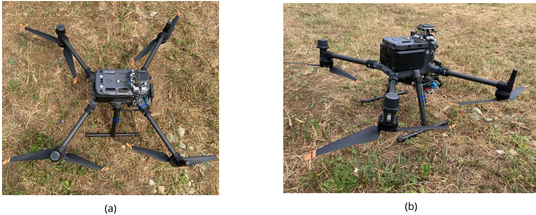
Figure 6.1: DJI Matrice 350 RTK with mounted multi-spectral camera: (a) Top view (left-hand side); (b) Front view (right-hand side).
