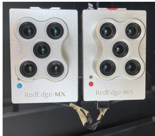
Figure 6.2: Two Micasense RedEdge MX Multispectral NDVI cameras that are mounted on the DJI quadrotor.
