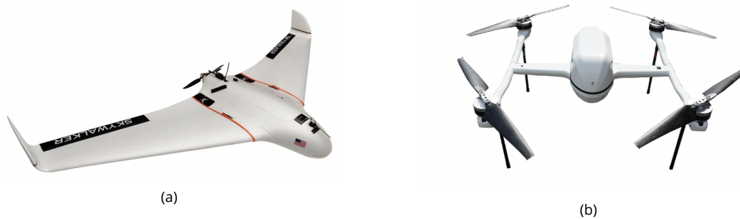
Figure 2.2: Wing-type classification of the UAVs: (a) Fixed-wing UAV; (b) Rotary-wing UAV (right-hand side).
