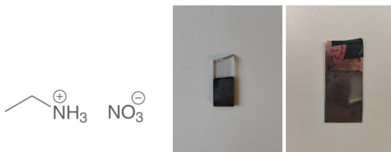
Figure 3.1 Formula of EAN and the deposition of the Ni-Co alloy on FTO glass and Cu foil.
