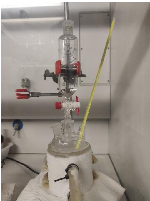
Figure 2.1 The synthesis of EAN.
