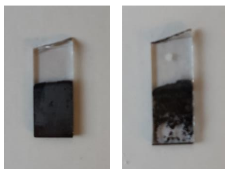
Figure 3.19 Photos of electrode before (left) and after (right) electrocatalytic testing.
