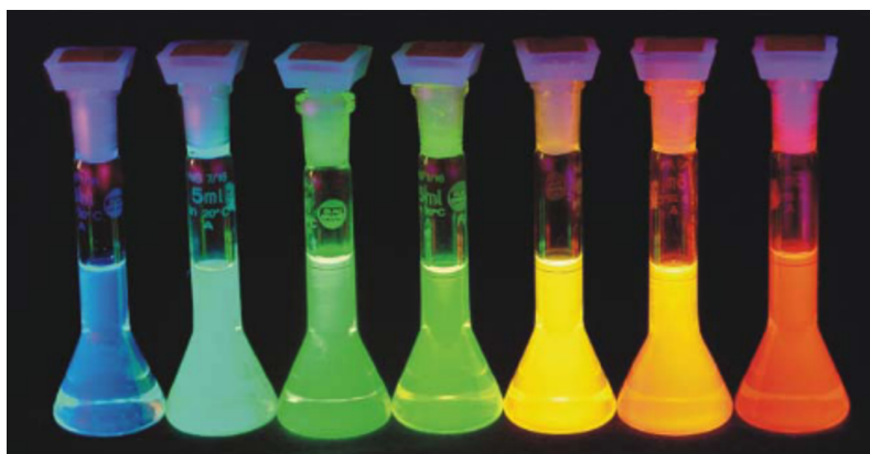
FIGURE 1.2: Fluorescence of CdSe/CdS core/shell nanoparticles with a diameter of 1.7 nm (blue) up to 6 nm (red), giving evidence of the scaling of the semiconductor band gap with particle size. Reproduced from the work of Roduner et al.[35]
