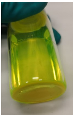
FIGURE 3.2: Picture showing the deposition of a precipitate in a typical micromolar oleylammonium-capped CsPbBr 3 colloidal dispersion.
