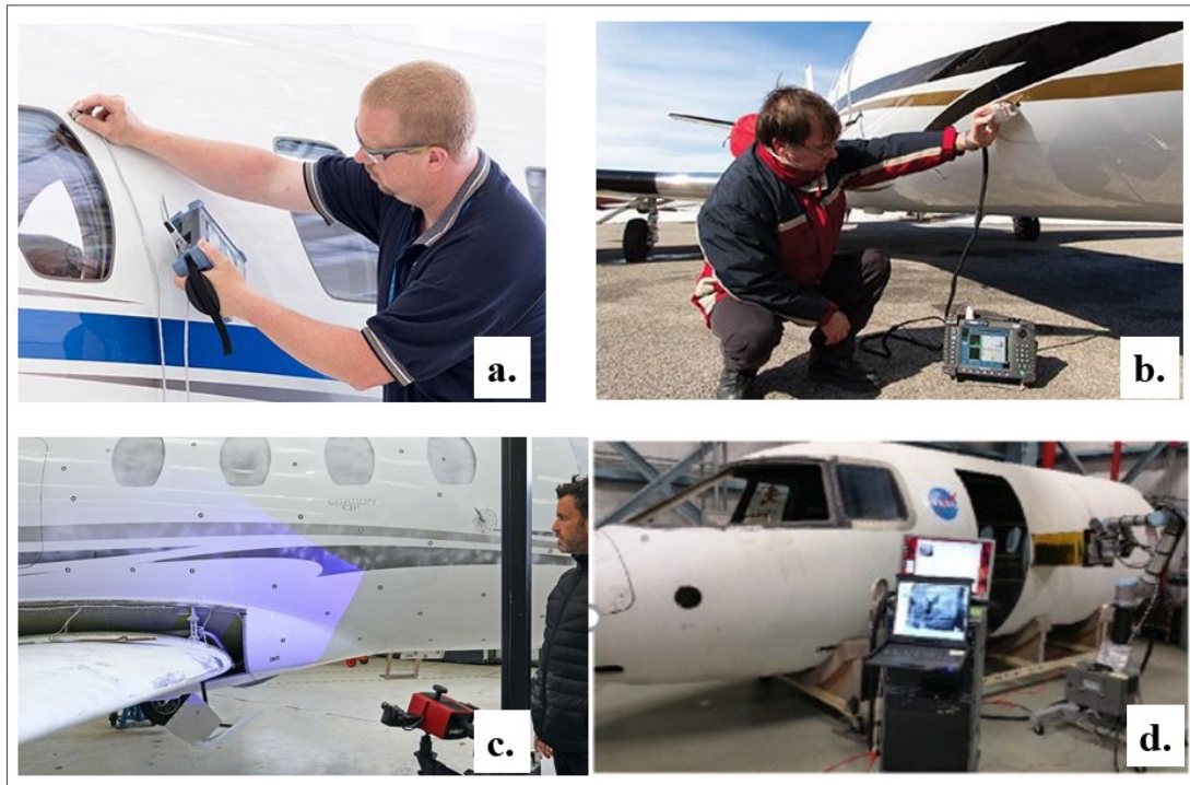
Figure 1.4: Illustration of NDT techniques currently applied in damage diagnosis of aerostructures, adapted from www.makepartsfast.com and www.gom.com .
