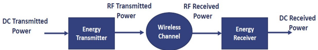
Figure 2.2: Wireless Power Transfer from DC to RF through an antenna transmitter to an antenna receiver.
