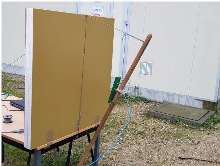
Figure 5.5: Receiving P2110b antenna along side the metallic plate.
