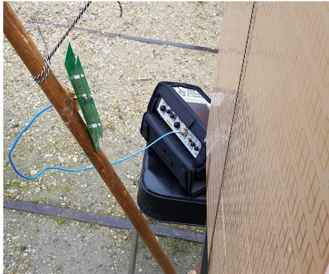
Figure 5.3: VNA to measure the received power by the Powercast P2110b dipole antenna.
