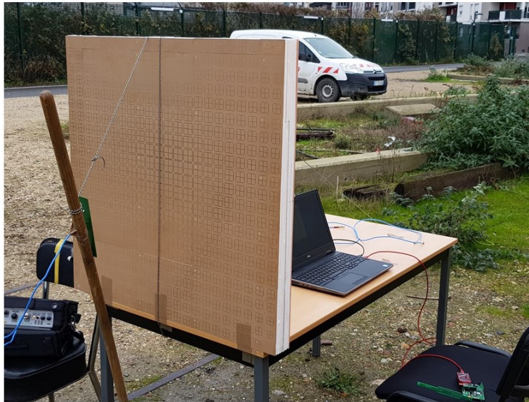
Figure 5.2: Setup of our focusing metasurface and harvesting device at a far distance from the railway system, including all components.
