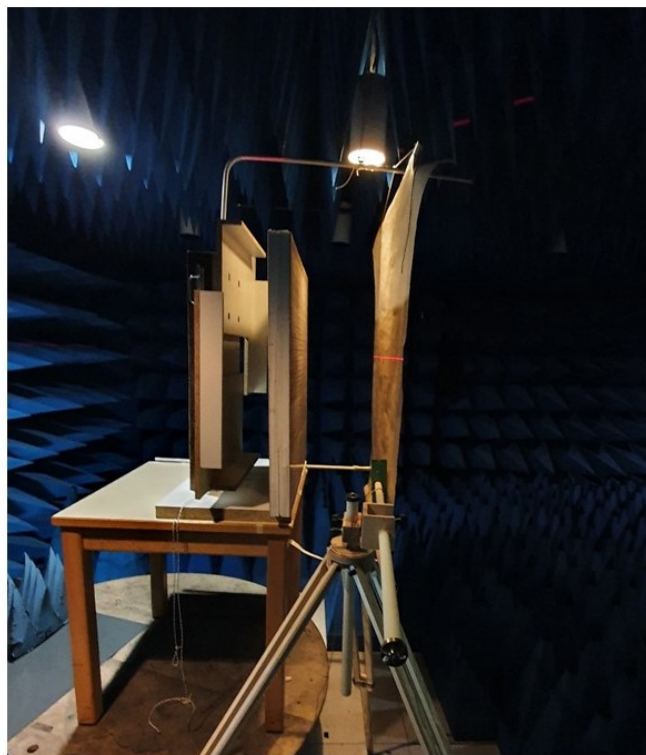
Figure 4.23: Dipole antenna measuring at each point 30 cm away from the metasurface at the fixed grid sheet.
