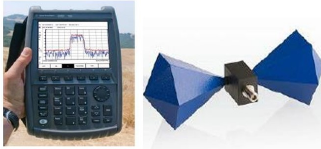
Figure 2.8: Spectrum analyzer and omnidirectional antenna for a band of frequency from 0.3 GHz - 3 GHz.(Imperial Colledge London)
