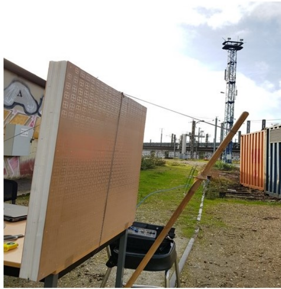
Figure 5.9: Setup of our focusing metasurface and harvesting device without facing the GSM-R base station in the far-field.
