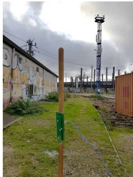
Figure 5.7: Receiving antenna implemented alone in the far-field away from the GSM-R base station.
