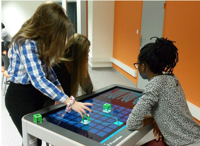
Figure 3.3: An example of the use of tangible tokens on an interactive tabletop: when in contact with the surface, the token becomes a controller to manipulate the virtual space (George et al. 2017)
