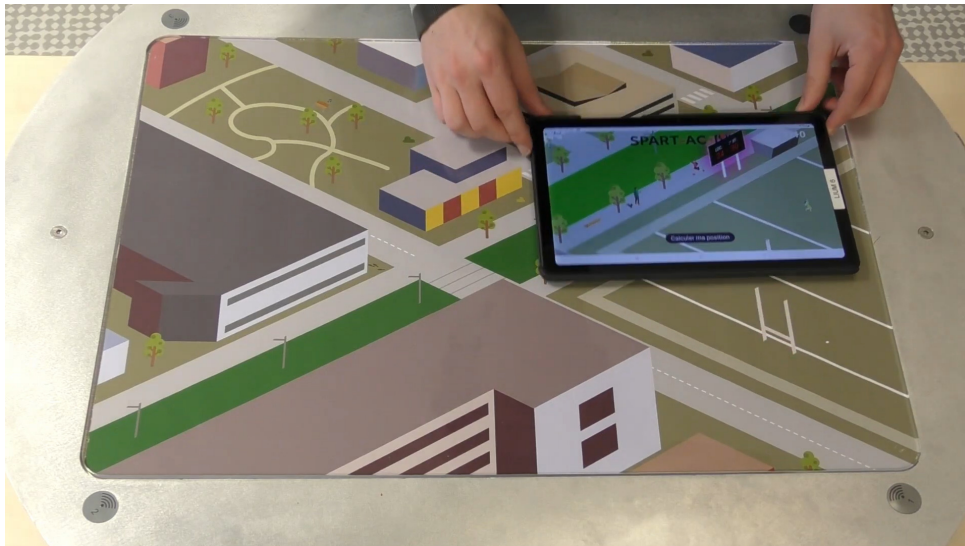
Figure 9.5: A photo of an acoustic prototype with four microphones and a mobile device as emitter
