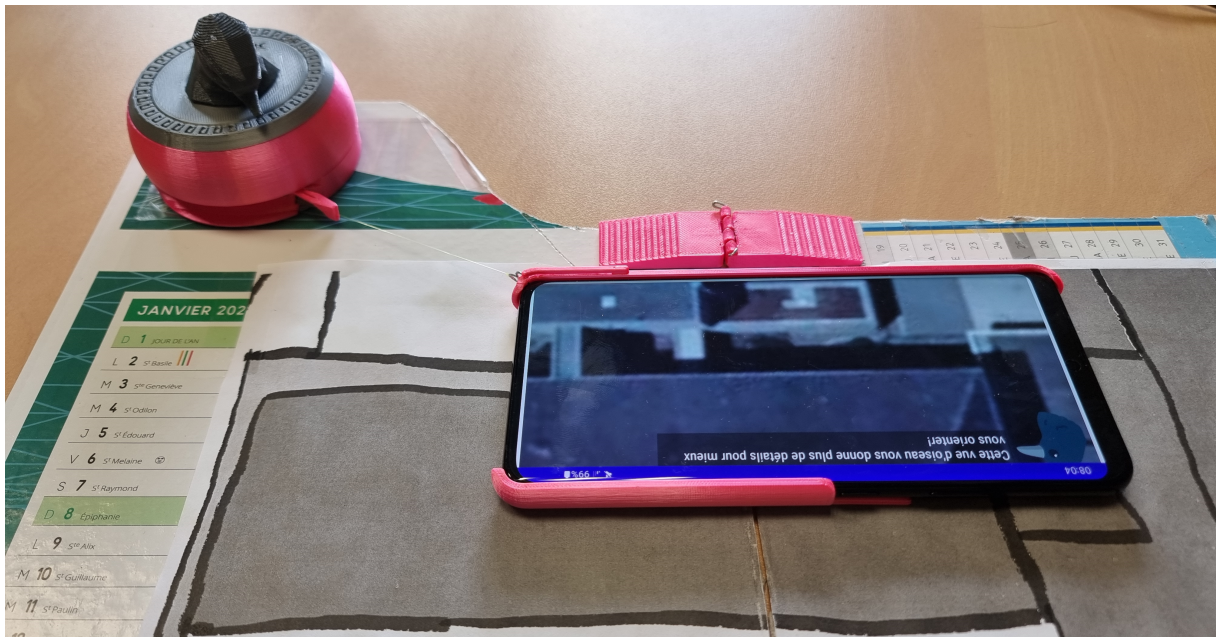
Figure 11.4: SPART-ME M with an NFC shield and the bird NFC token, unlocking a satellite image view on the connected smartphone
