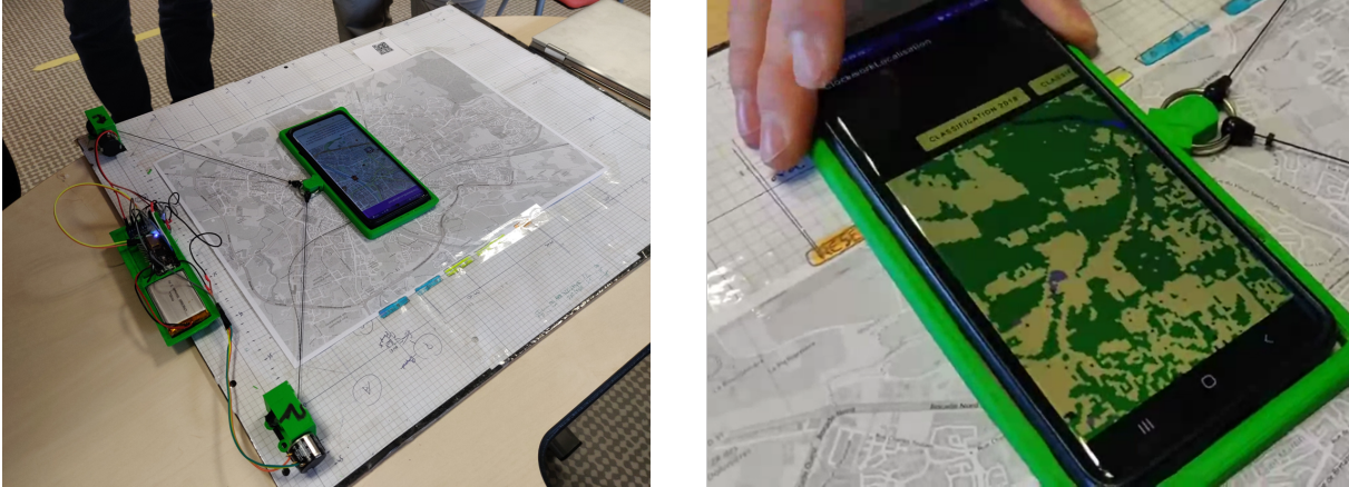
Figure 9.6: SPART-ME D (Dual String)- left: potentiometers and strings with microcontroller, right: zoom on augmented content
