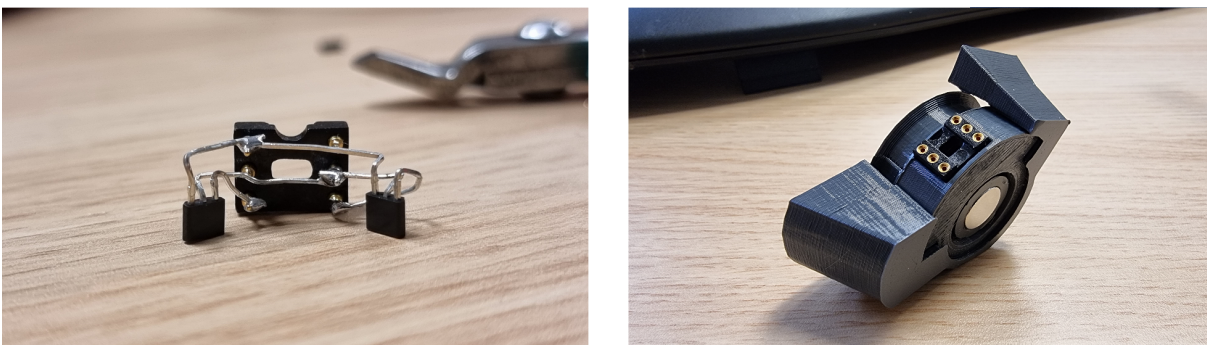
Figure 9.12: Soldering of two S49E Hall sensors (left) for use in the assembled rotary encoder (right)
