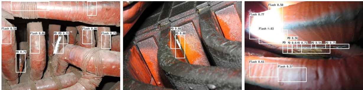
Figure 4.11: Some results of PD and reflected flashlight detected by the Faster-RCNN model.
