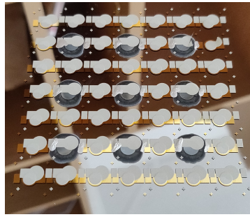
Figure 4.21: Wafer with the top electrode screen-printed with a silver ink.
