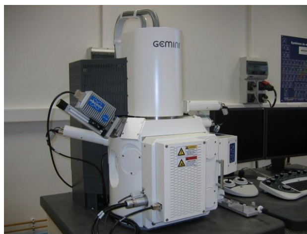
Figure 65: Scanning Electron Microscope set-up (left) besides its display set-up (right) at LEDNA facility, CEA Saclay
