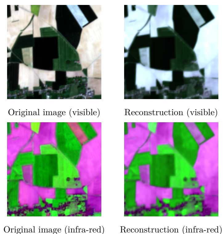
Figure 8.9: S2 region of interest (ROI) image from test data-set acquired on 2023-05-13 and located at T31UFS tile (Southern Belgium). First column shows true and false color composites constructed by original S2 reflectance values whereas PROSAIL-VAE reconstruction results are displayed at the second column. The red green blue (RGB) true color composite corresponds to bands (B4, B3, B2). The RGB false color composite corresponds to bands (B11,B8,B5)
