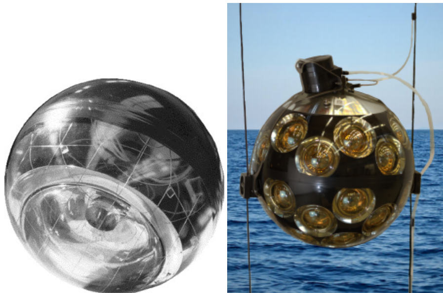
Figure 4.16.: Left: ANTARES Single-PMT optical module. Right: KM3NeT Multi-PMT optical module.
