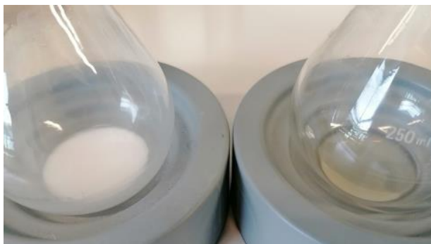
Figure 5.2. Image of 5/5 w/w PAA-PDADMAC polymer complex in miniemulsion (left) and nanosuspension (right) prepared via two-step emulsification and evaporation method reported in Table 5.2 (sample 11).
