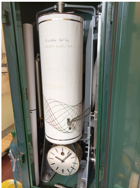
Figure 8.4: Photos taken during a visit of the SHOM, Brest, March 2024. Left: former Port-Tudy tide gauge. Right: current Brest tide house, with tide staff on the wall.
