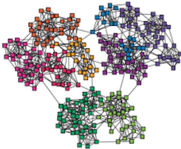
Figure 2.5 – Example of a graph partitioned into 7 communities. Nodes of the same color belong to the same community
