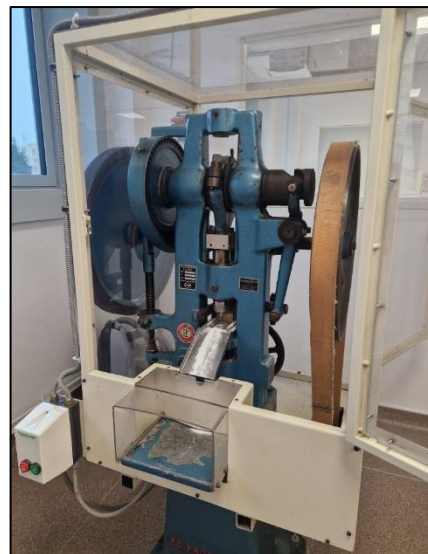
Figure 55 : Machine de compression FROGERAIS
