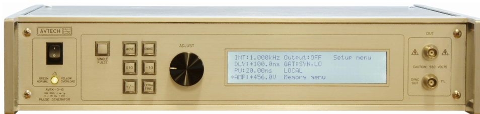
Figure 2.7: Front side of the Avtech Electrosystems Ltd. AVRK-4-B High Voltage Pulser, used during all my thesis experiments.
