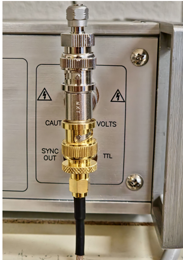
(a) Actual implementation of the proposed impedance matching.
