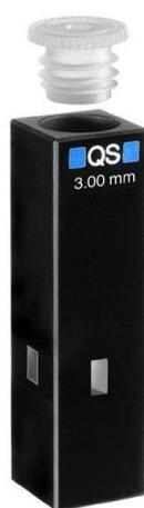
*Figure IV-8: 200  $\mu$ L Quartz Fluorescence cuvette. The cuvette used for the quenching experiments.*
