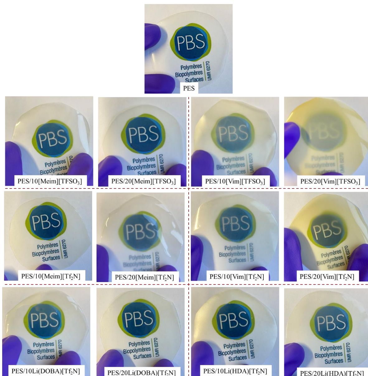
Figure 4-1 Optical photos of PES and PES/ILs membranes
