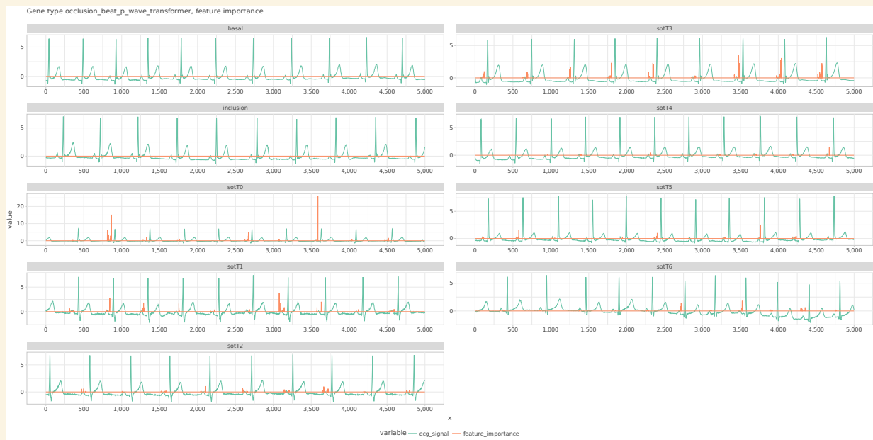
Figure 33: Experiment 2 - Features importance P Wave: features importance computed using integrated gradients method.
