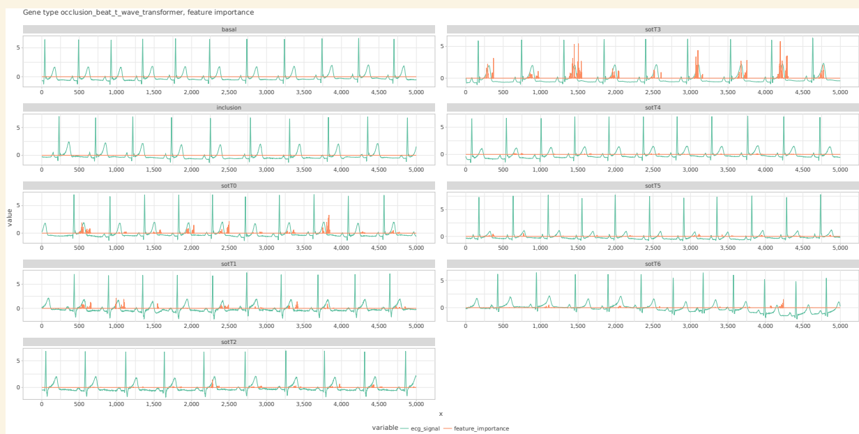
Figure 34: Experiment 2 - Features importance T Wave: features importance computed using integrated gradients method.
