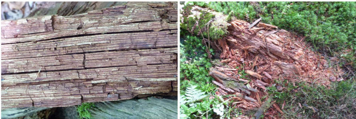
Figure I-7 - Wood degraded by brown or cubic rot fungi (left) and soft rot fungi (right) [18]
