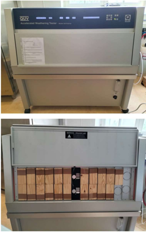
Figure 0-5 - Photos of the equipment used (left) and illustration of the inside of the QUV (right)
