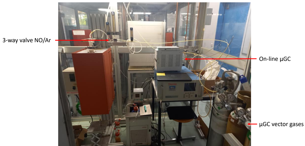
Fig. 1.12. Scheme and picture of the setup for deNO x experiments, 2 nd campaign
