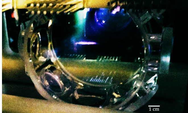
FIGURE 2.6: Fluorescence of cesium atoms inside the elongated magneto-optical trap. The fluorescence of cesium atoms is represented by the bright area at the center of the vacuum chamber.
