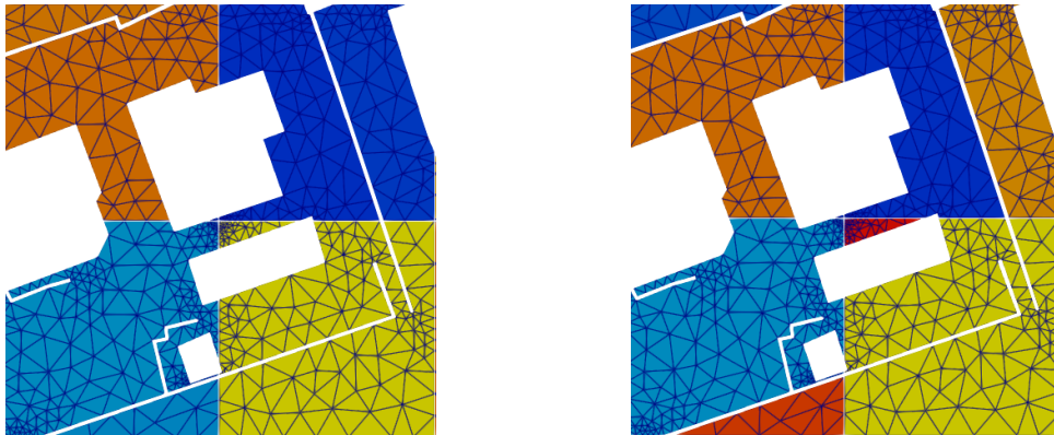
Figure 2.4: Possible partitioning of the domain without (left) and with (right) additional partitioning by disconnected component, with each subdomain/component depicted by a color block.
