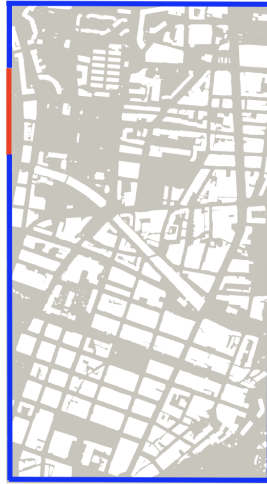
Figure 3.6: Boundary condition (thick blue and red lines) and corresponding model domain for Example 3. Red corresponds to u = 21.5 meters, blue corresponds to u = z_b . This results in around a 2-meter elevation for the portion of the boundary representing the Paillon river.
