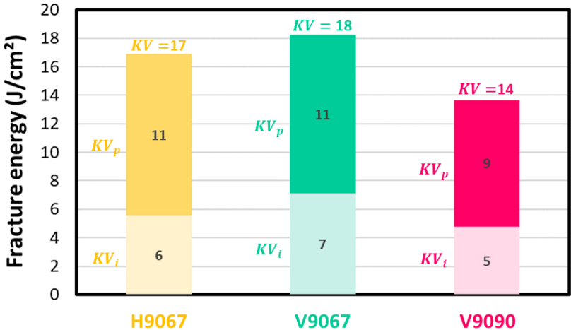
Figure 83: Mean fracture energies obtained during impact tests for all configurations (Fracture energy at initiation KV_i , during propagation KV_p , and in total KV)
