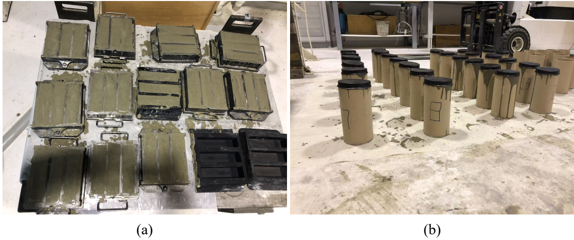
Figure 2.1 Prismatic specimens in Part I and II (a) and cylindrical specimens in Part III (b) cast in plastic and paper molds.
