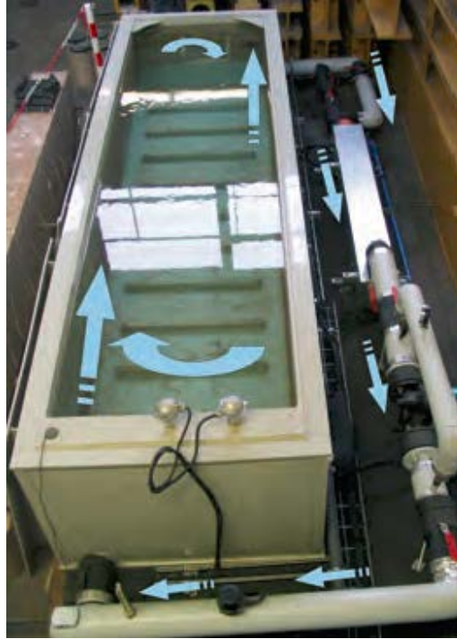
Figure 2.3 Bath with a heating device using in this study.
