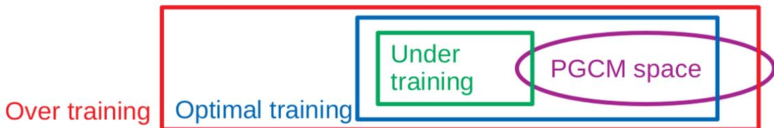
Figure 7.3: Schematic illustration of the three training regimes. At first, the (P)GCM subspace corresponding to a given simulation (purple) is imperfectly reproduced by a too small training space (green). In a second phase, the emulation of the (P)GCM subspace constitutes an optimal compromise (blue). Eventually, the (P)GCM subspace is well emulated at the price of a too large training space inducing a non-negligible over training (red).
