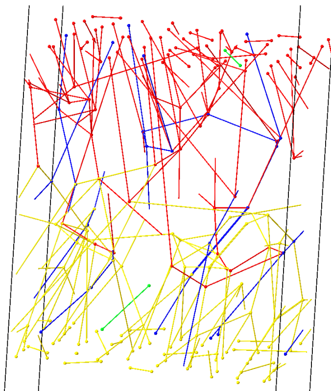
Figure 4.3: The primitive paths of chains in an amorphous region computed with the Z1 code [Kröger, 2005], the segments belonging to loops are yellow and red, the segments belonging to tie chains are blue, the tail segments are in green. The spheres represent the primitive path kinks and the ends of the chains.
