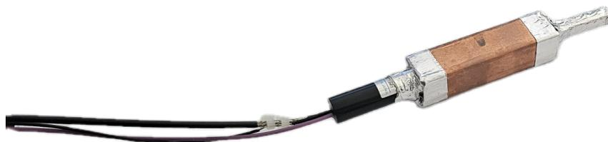
FIGURE 3.11 – The small solid angle plastic scintillator used during the experiment. It was placed on top of the HPGe aluminum cap and held in place using tape.
