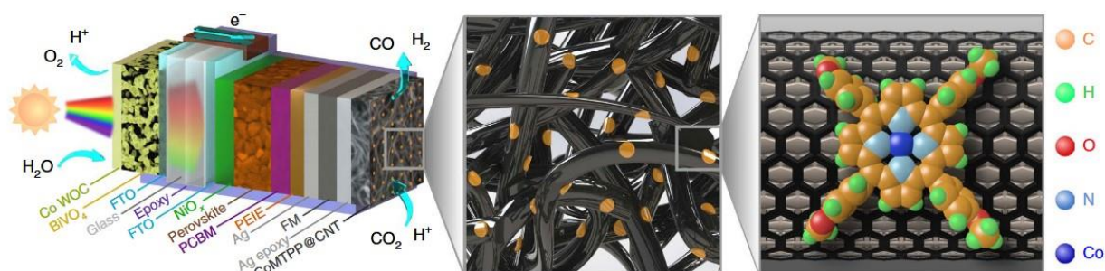
Figure 1.8 Architecture of the standalone perovskite–BiVO 4 PEC tandem device for bias-free syngas production. Oxygen evolution occurs at the front BiVO 4 photoanode with a Co WOC. An inverse-structure perovskite photocathode reduces CO 2 and protons to CO and H 2 via a CoMTPP molecular catalyst immobilised on a CNT sheet. An embedded copper wire connects the two photoelectrodes in this artificial leaf configuration. 44
