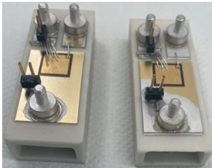
Figure 5.34: Soldered power connectors and auxiliary pins for the connection to the outside world.
